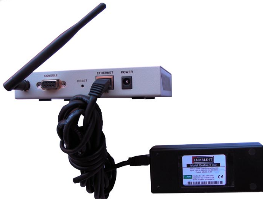
Figure 1 Enable-IT 350 to a 8424 WiFi PoE Access Point
